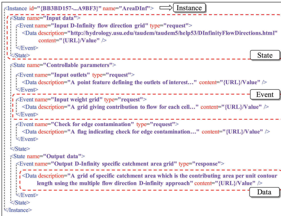
Figure 3. Structure of a typical data I/O configuration document; there are four basic XML nodes: Instance, State, Event and Data node.
